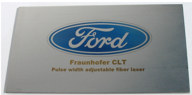
Figure 11. Laser color marked logo on Titanium.
