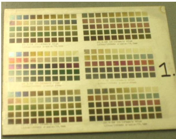
Figure 6. Set of parameter matrixes marked using 100 and 125 ns pulse width.
