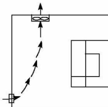
Correct installation position of the fan
