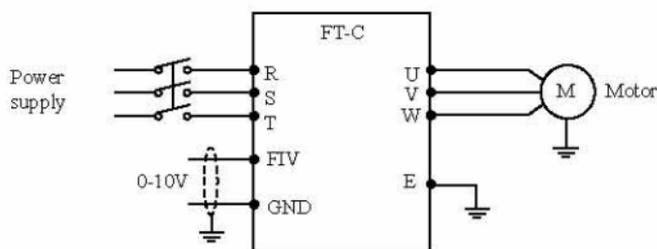
Explanation: control the output frequency through terminal FIV/ FC (0~10V).
