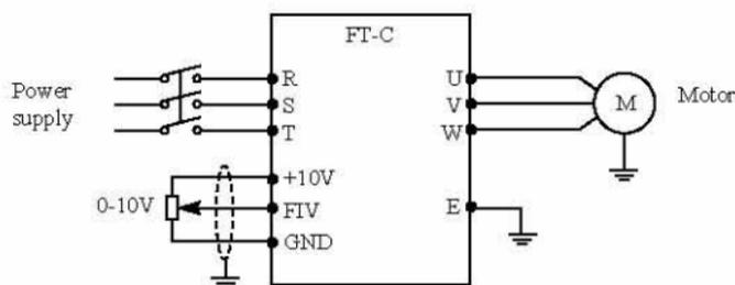
Explanation: control output frequency of inverter by FIV voltage signal sent by external POT (10k  $\Omega$ )
