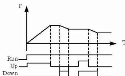
Explanation: when UP is valid (UP is closed), frequency will go up. When DOWN is valid (DOWN is closed), frequency will go down.
