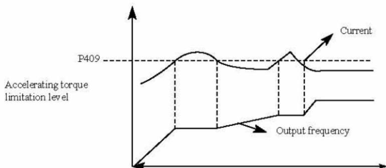
100% current is the rated current of inverter, when P409 is set to be 0, then accelerating torque limit is invalid, and it does not have protecting function.
