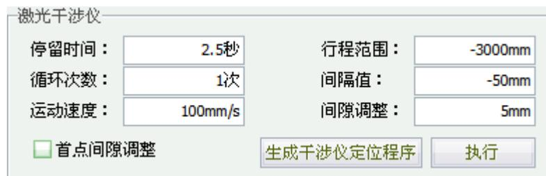
Herein, the travel range is automatically read, please set as same as the setting value of the interferometer, but pay attention to symbols. Input a negative value when forward home origin, whereas input a positive value. If input an error value, the system will prompt when you save.
